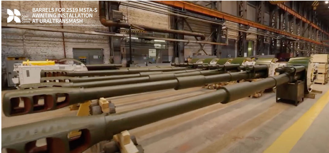
Figure 4: Cannon units for Msta-S, made by Volgograd-based Titan-Barrikady Plant, 22 ready for assembly at Uraltransmash in Yekaterinburg, April 2023
